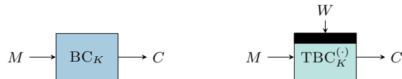
Fig. 15: Block-cipher (left) and tweakable block-cipher (right). For tweakable block-ciphers, the black bar indicates that the incoming arrow ( W ) is the tweak.
