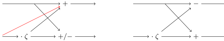
Fig. 1. Butterfly operation of [48] (left) vs Cooley-Tukey’s [21] (right); in red the extra addition.
