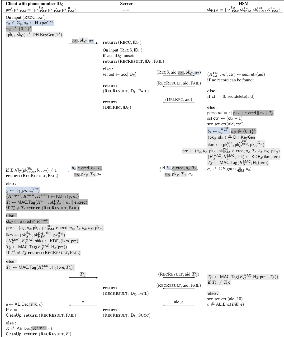
Figure 5: The WBP key recovery. Light blue boxes indicate 2HashDH instructions of OPAQUE; light gray boxes mark 3DH of OPAQUE; dark gray boxes denote other OPAQUE instructions; non-colored parts were added by WhatsApp. \xrightarrow{a} is the ID_C -authenticated transmission of a .
