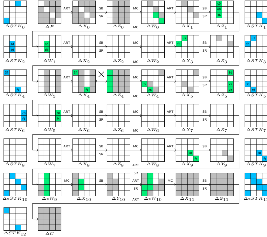
Figure 13: 12-round related-tweakey impossible differential attack against Deoxys-BC-384
