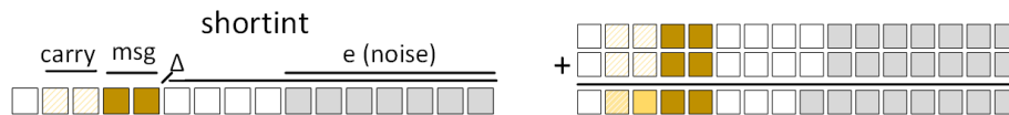
Fig. 4: (left) TFHE Shortint Ciphertext of 2-bit message : This is a visualization of a TFHE ciphertext, where each square represents one bit. The illustration shows that the TFHE message bits are encoded in the upper bits, with noise added to the lower bits; (right) Addition of Two Ciphertexts : This figure shows an sample operation. Both the message size and noise grows; note that if too many operations are performed, the noise will start overwriting the message bits and corrupt the output. Noise can be reset with a bootstrapping operation.
