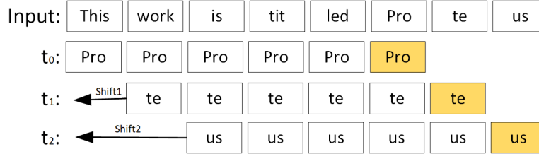
Fig. 7: Homomorphic String Comparison: This figure illustrates homomorphic string comparison with the tokens {"Pro", "te", "us"}.
