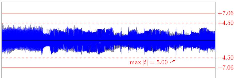
**Fig. 7.** 100,000 traces of the core signing process (5.95M cycles, one sample per cycle at 31.24MHz). The TVLA test had a maximum spike of  $|t| = 5.00$ , which is below the long-trace adjusted critical value  $C = 7.06$ .
