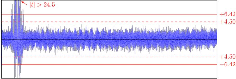
**Fig. 6.** A TVLA test of a processor implementation of SLH-DSA rapidly shows a leak of SK.seed secret key material. In this  $t$ -trace we captured the initial 73k cycles of the signing process, containing the first SHAKE256 PRF call. Maximum  $t$  value reaches 24.5 already in 1,000 traces. The SHA2-256 PRF exhibits similar leakage behavior.
