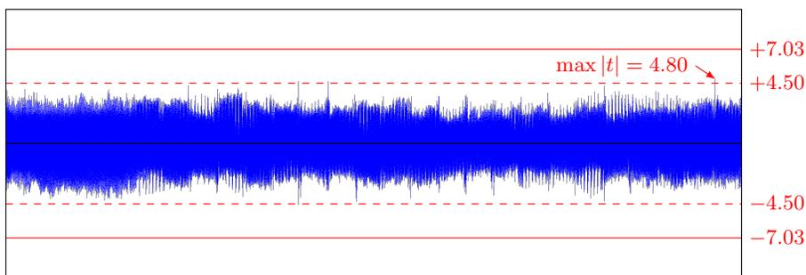
**Fig. 8.** 10,000 traces of the core signing process (SLH-DSA-SHAKE-128f) has a maximum spike at  $|t| = 4.80$ , which is below the critical value  $C = 7.03$  with 4.91M time points. The secret keys are entirely handled by hardware, reducing their exposure to side-channel attacks.
