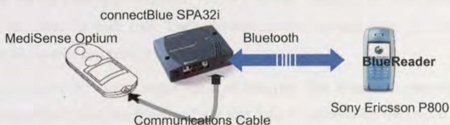
Figure 60. MDMIS Experimental Set-up Test for the Bluetooth Connection Evaluation
