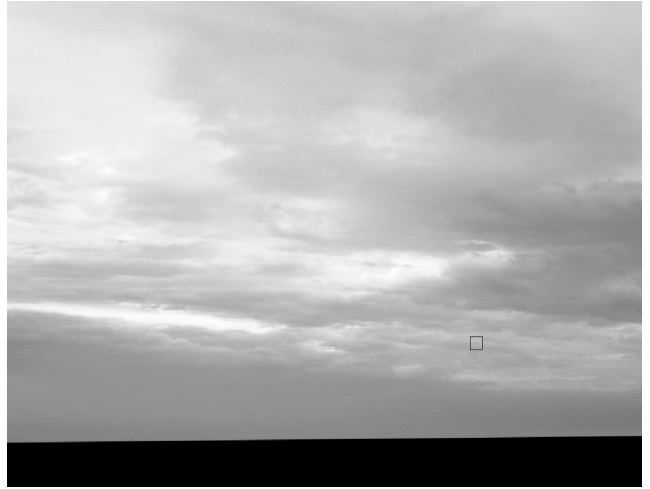
Fig. 5. Illustrative image frame from encounter 14 just after target is detected (frame 790). The black region at bottom of the image is a result of image stabilisation. The location of the detected target is shown by the black box.
