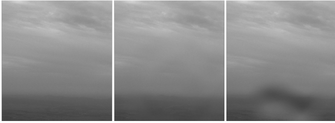
Fig. 4. Effect of the rain drop in three consecutive frames: no drop on the left image, circular shaped drop contacted the lens in the centre, drop disappearing due to airflow on the right image. Encounter 15.
