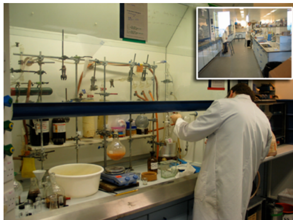
Figure 3. A fume cupboard in a chemist's laboratory. Inset, the distance between the fume cupboard and the bench.
