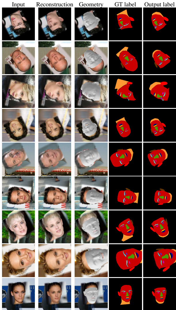
Figure 9: Reconstruction results based on CNN trained with semantic label loss and photometric loss.
