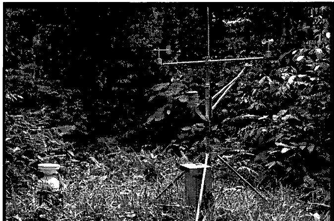
Plate 2.4 The ARG100 0.2 mm tipping bucket raingauges for gross rainfall measurement in the logged-over area (front left). The automatic weather station for microclimate measurements is in the centre.
