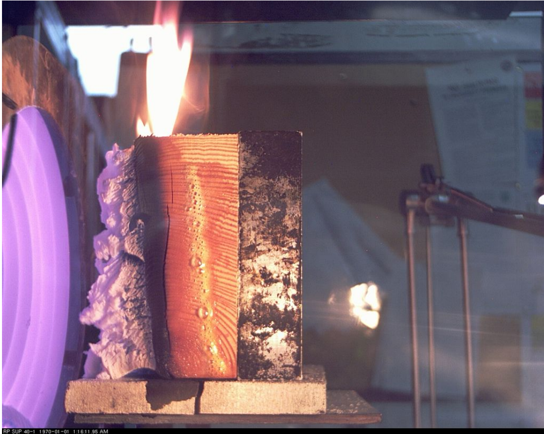
Figure 3.5: 3950 s: transition to flaming. Pulsating flame is first observed on the top portion of the sample. Note the how the moisture evaporation front is now at an angle with respect to the exposed surface. This is caused by the insulating effect of the ceramic fibre board on the bottom of the sample. Sample is exposed to an incident heat flux of 40 \text{ kW}\cdot\text{m}^{-2} , perpendicular heating.
