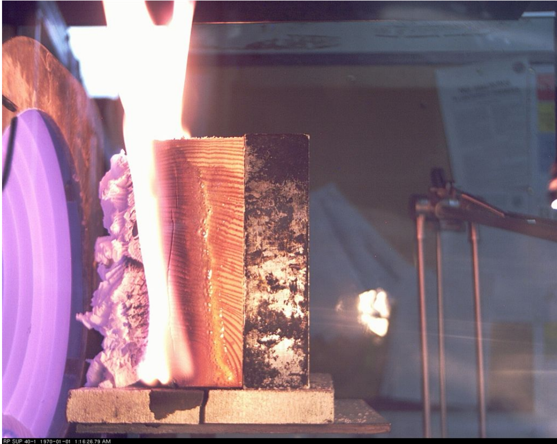
Figure 3.6: 3965 s: flame descends to the sides of the sample. Pulsating flame now is located over the pyrolyzed parts of the wood. Sample is exposed to an incident heat flux of 40 \text{ kW}\cdot\text{m}^{-2} , perpendicular heating.
