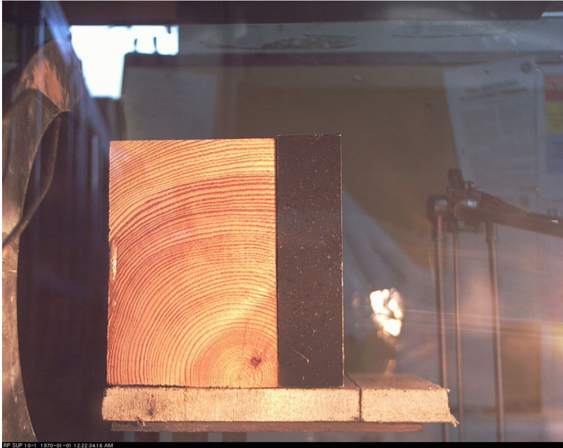
Figure 2.4: Photograph of a specimen during a test. The cone heater is located at the left of the photograph. The aluminium block is seen at the right of the sample, while the white object underneath the wood specimen is the ceramic fibre insulating board.
