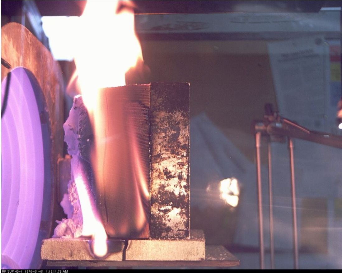
Figure 3.7: 4070 s: whole sample is involved in flaming. The charring front has advanced until the back end of the sample, and the moisture evaporation front is not noticeable. Sample is exposed to an incident heat flux of 40 \text{ kW}\cdot\text{m}^{-2} , perpendicular heating.
