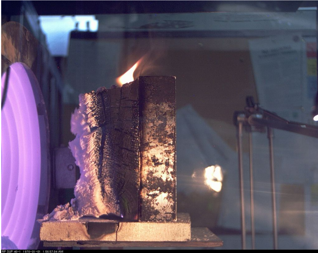
Figure 3.8: 6395 s: flaming about to end. The char oxidation is more important at the base of the sample, due to the insulating effect of the ceramic fibre board. The test is about to end. Normally the temperature profile tests are stopped when the thermocouples read temperatures above 873 K. Sample is exposed to an incident heat flux of 40 \text{ kW}\cdot\text{m}^{-2} , perpendicular heating.
