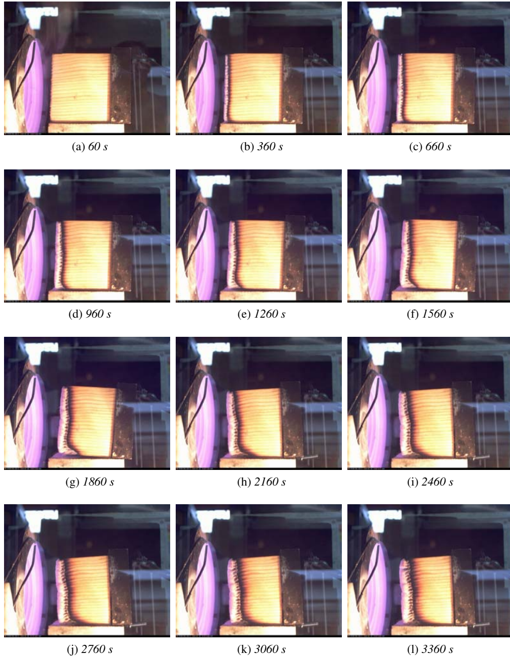
Figure B.10: 60 \text{ kW}\cdot\text{m}^{-2} , parallel heating. Charring and surface oxidation fronts evolution in time. Note the insulating effect of the sample holder, which accelerates the reactions at the bottom of the specimen and the absence of the moisture evaporation front, due to a lower diffusivity in the transverse direction (perpendicular to the grain).
