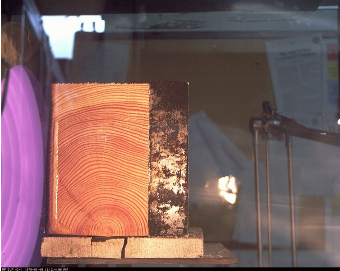
Figure 3.3: 140 s: maximum mass loss rate is attained at this time. The moisture evaporation front corresponds to a lighter coloured line on the left side of the sample. At this instant the front is parallel to the exposed surface. Sample is exposed to an incident heat flux of 40 \text{ kW}\cdot\text{m}^{-2} , perpendicular heating.
