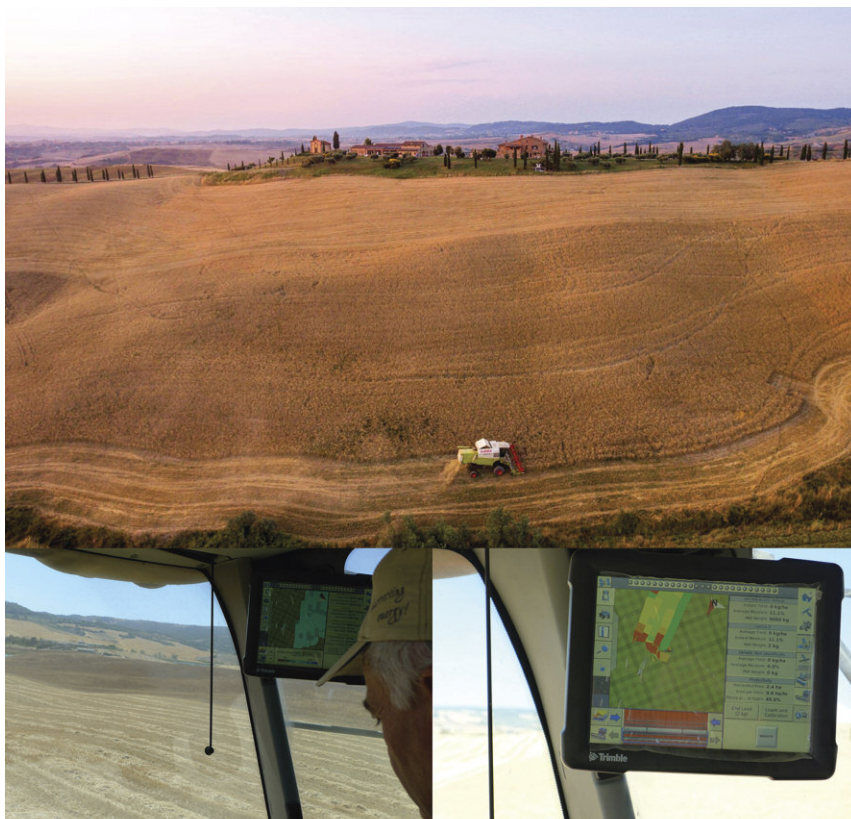
Figure 1: Combines equipped with yield monitoring sensors for measuring and recording information such as grain flow and moisture, area covered and location.
