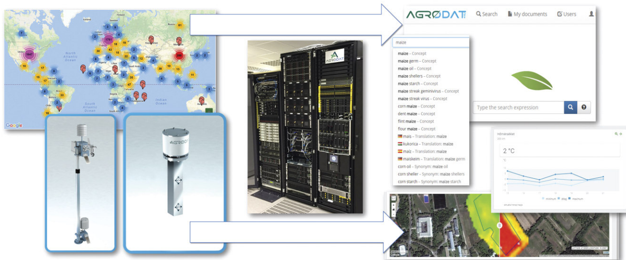
Figure 1: High-level concept of Agrodats: data sources + Big Data centre + decision support system with knowledge base/multilingual search engine.
