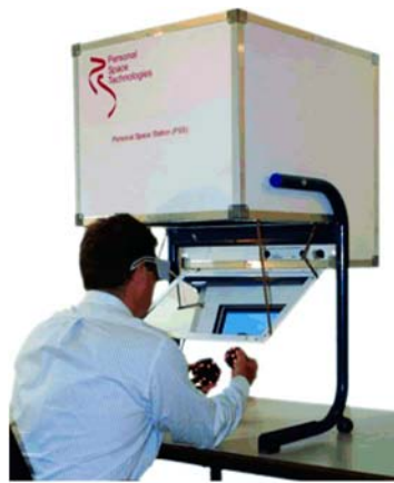
Figure 1: The PSS explained. In the PSS the user holds the image in his hands and manipulates it with tangible interaction devices. The user looks at the monitor via a mirror. This enables the user to bring his hands into the same environment as the virtual 3D-objects without interrupting the visual image. With the use of a custom optical tracking system, the user can interact with the 3D images using wireless, tangible interaction devices. Therefore, interaction with virtual objects can take place in a direct, natural and intuitive way. Hand-eye coordination and 'proprioception' (the subconscious perception of the position of muscles and joints) are used to the full. The user is 'attracted' by the objects he sees; his natural reaction is usually to grab and manipulate them.
