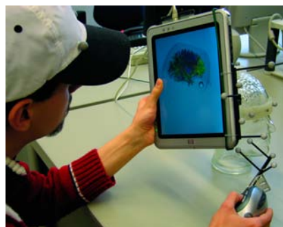
Figure 2: A position-tracked interactive display for the co-located visualization of medical images and simulation results. Displays like this can be a powerful planning and navigational tool in surgical treatments. Picture: UvA.
