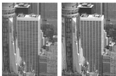
Figure 2: Aliasing reduction with a post-decompression filter.
