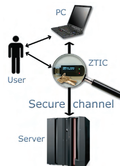
Figure 1: The secure channel is opened between the (bank's) server and the ZTIC. The user communicates as usual with the server via a PC.
