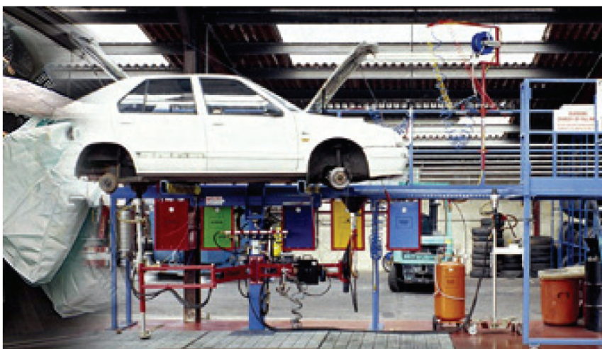
Figure 2. A dismantling station – removing dangerous waste materials.
