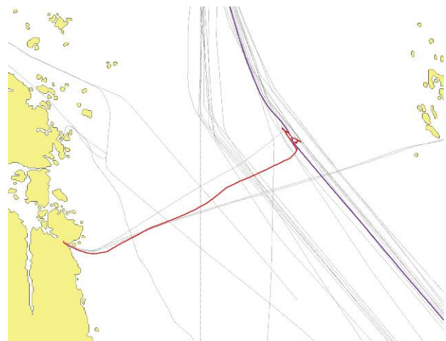
Figure 2: A small fishing boat (red) repeatedly stopped in the middle of the shipping route. It was almost hit by a large freight ship (purple).
