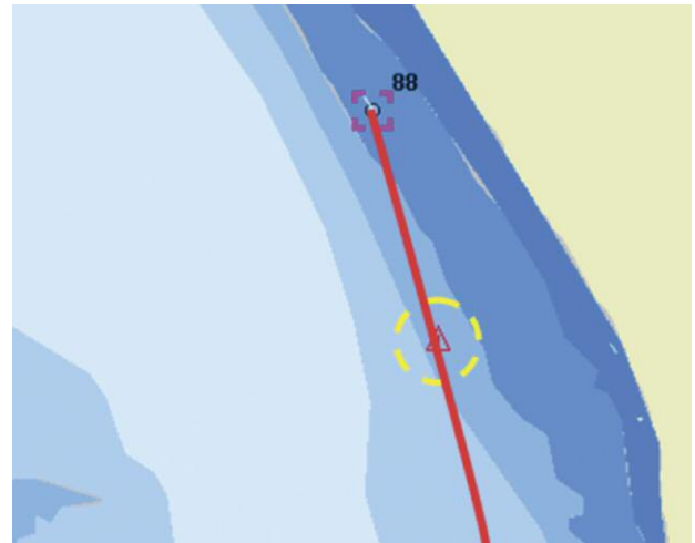
Figure 1: The risk of grounding was detected (yellow ring) three minutes before it actually occurred (purple square).
