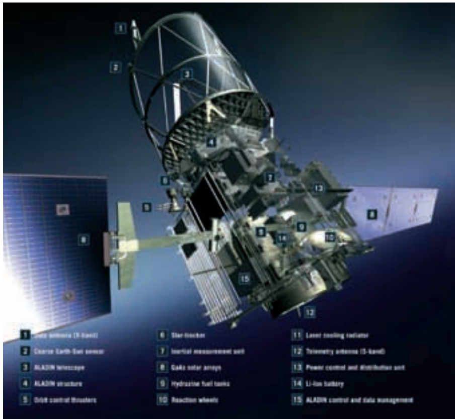
Fig. 4.34. X-ray view of the Aeolus satellite, indicating the key satellite subsystems.
