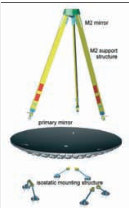
Fig. 4.22. Exploded view of the lightweight transmit-receive telescope in SiC technology. M1: primary mirror of 1.50 m diameter, M2: secondary mirror, I/F: interface, ISM: isostatic mounting structure, MS: mounting structure. Courtesy of Astrium Satellites SAS.
