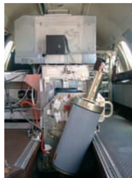
Fig. 6.4. The ALADIN Airborne Demonstrator – A2D – inside the DLR Falcon 20 during test flights in October 2005. Courtesy of DLR.
