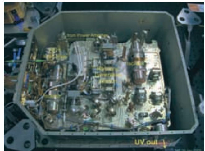
Fig. 4.20. Power Laser Head Lower Optical Bench (LOB) carrying the passive elements. The LOB is seen in the laser housing, with the lid open. Photo courtesy of Galileo Avionica
