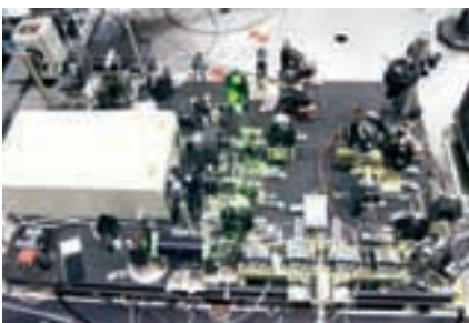
Fig. 4.38. ALADIN signal simulator OGSE set-up, showing the continuous wave Nd:YAG laser with a tripling stage, a set of four acousto-optical modulators for frequency tuning and an electro-optical modulator for intensity modulation of the UV beam. The signal is coupled into an optical fibre to guide it into the ALADIN test chamber.
