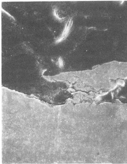
Fig. 10. Cross section of 310SS eroded surface showing platelets.
