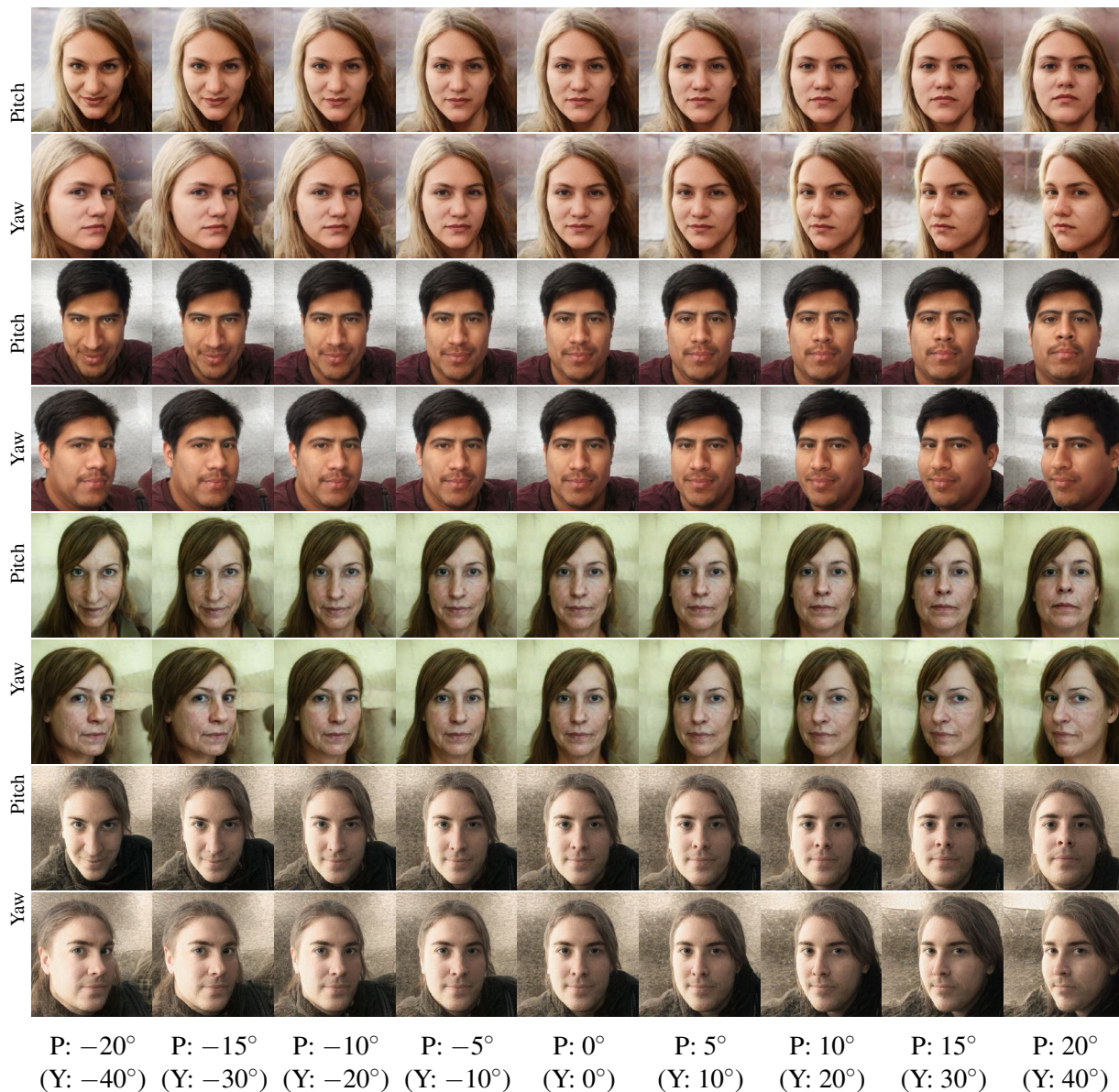
Figure 3.9: Head Redirection Results. The gaze directions are all set as (0^\circ, 0^\circ) . ‘Pitch’ (P) means that we only redirect the pitch component of head orientations and set yaw as 0^\circ . ‘Yaw’ (Y) means that we only redirect the yaw component of head orientations and set pitch as 0^\circ . The redirected angles are listed at the bottom of the figure.
