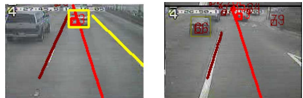
Fig. 16. Preliminary sensor-fusion result of vision-based lane-and-obstacle-detection results, LIDAR, and vehicle navigation information. The obstacles' relative positions with respect to the lane are estimated. The thick red line is a projected vehicle path.
