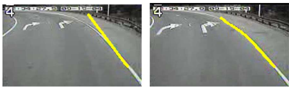
Fig. 14. Misalignment corrected by redundant detections in the following frames.
