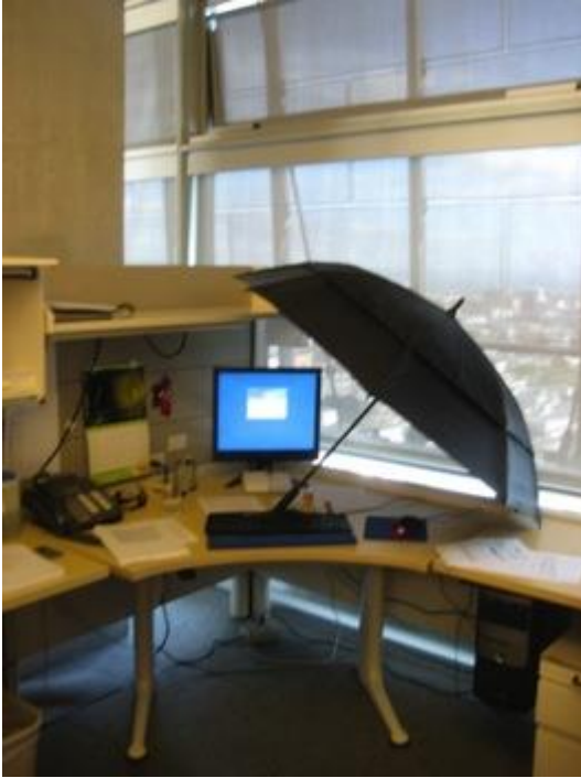
Fig. 27. Example of personal workspace modification on the SE facade to block direct view of the solar disc.
