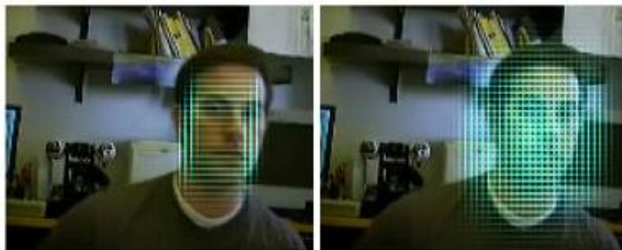
Figure 3.5: An example of uncertainty propagation: The left side shows the most probable hypotheses at time t , i.e., the filtering distribution. The image on the left shows the predictive distribution for time t + 1 , i.e., the prior distribution for the next time step.
