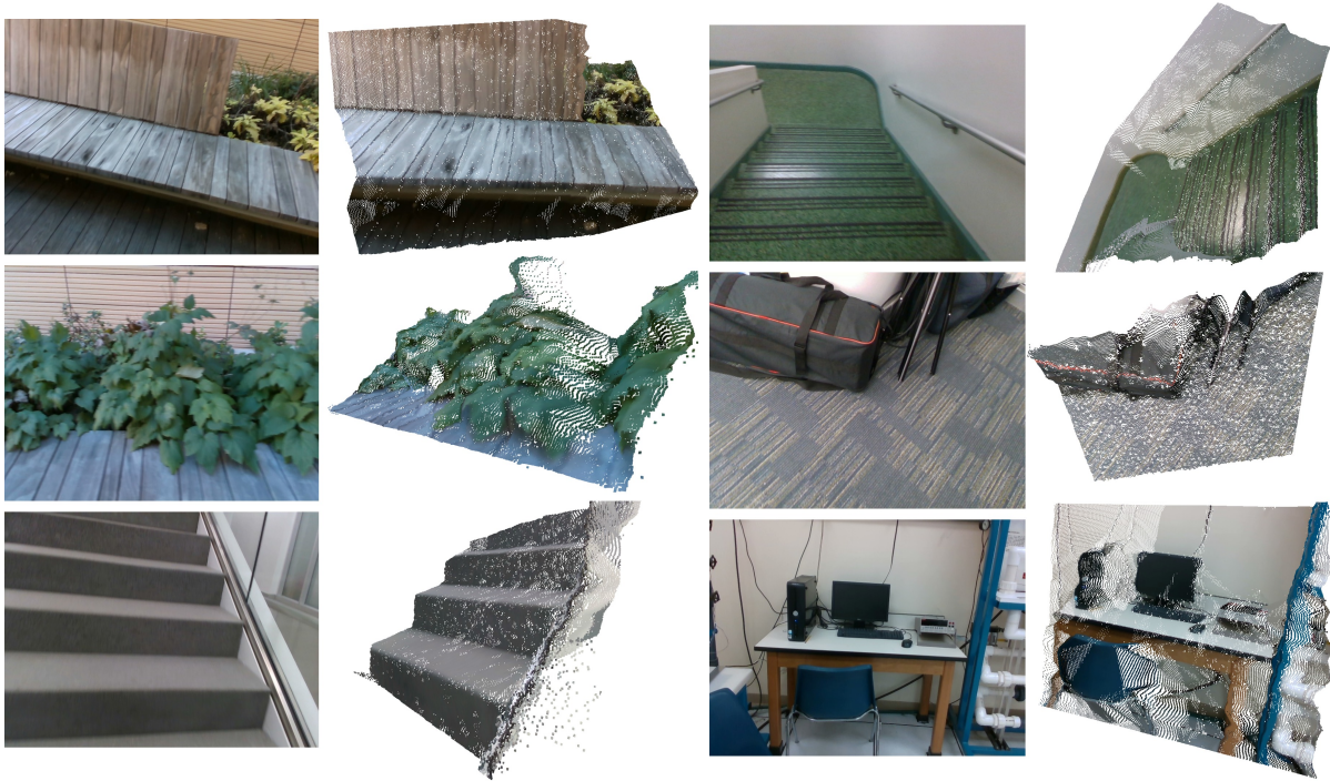
Figure 3.7: More Qualitative results on VOID dataset. In each panel, the left shows a sample RGB image fed to our depth completion network as input; the right shows the completed depth map back-projected to 3D, colored, and viewed from a different vantage point. Our method recovers the scene structure with details at various ranges in both indoor and outdoor settings.
