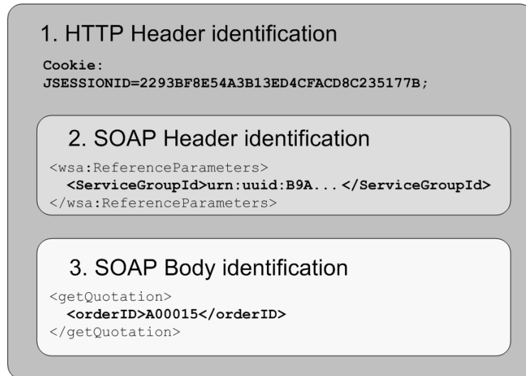
Figure 10 – Identification information can be supplied in three different layers of service requests
