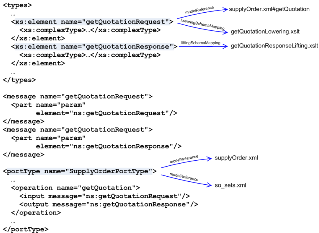
Figure 36 - SAWSDL annotations of the SupplyOrder WSDL file with model references and schema mappings
