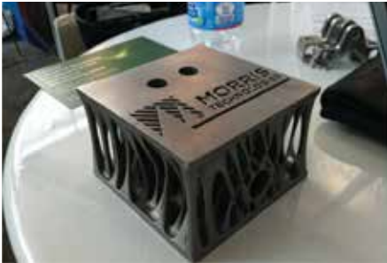
Morris Technologies 3D printed metal aerospace part. Photo: S. Boisvert, courtesy of Greg Morris. ??
