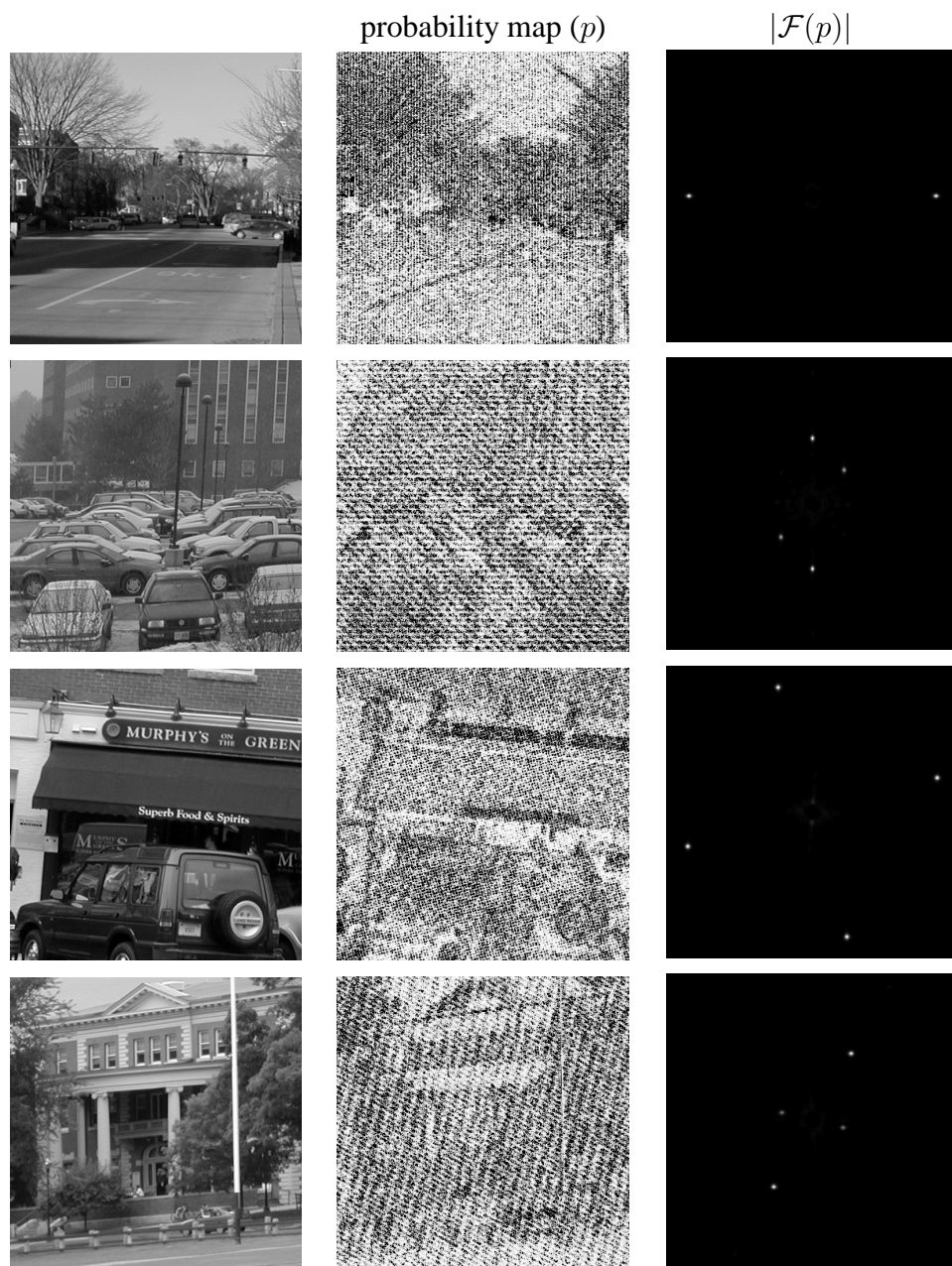
Figure 2.7: Shown in the left column are four images affine transformed by random amounts. Shown in the middle column are the estimated probability maps ( p ) that embody the spatial correlations in the image. The magnitude of the Fourier transform of each map is shown in the right-most column. Note that these images yield periodic maps.
