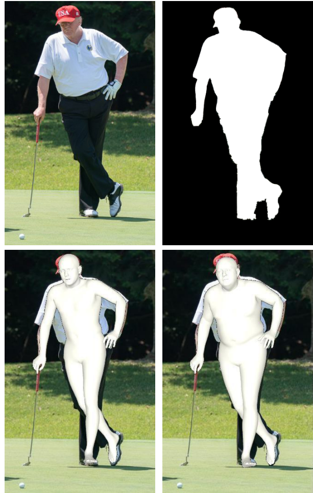
Figure 2. An input image and manually extracted binary silhouette (top row). A fitted 3D SMPLX model without (bottom left) and with (bottom right) the additional silhouette-based, body-shape constraint. Although body pose is well estimated in both cases, the additional constraint yields a more accurate estimate of body shape. [photo source: Official White House Photo by Shealah Craighead]
