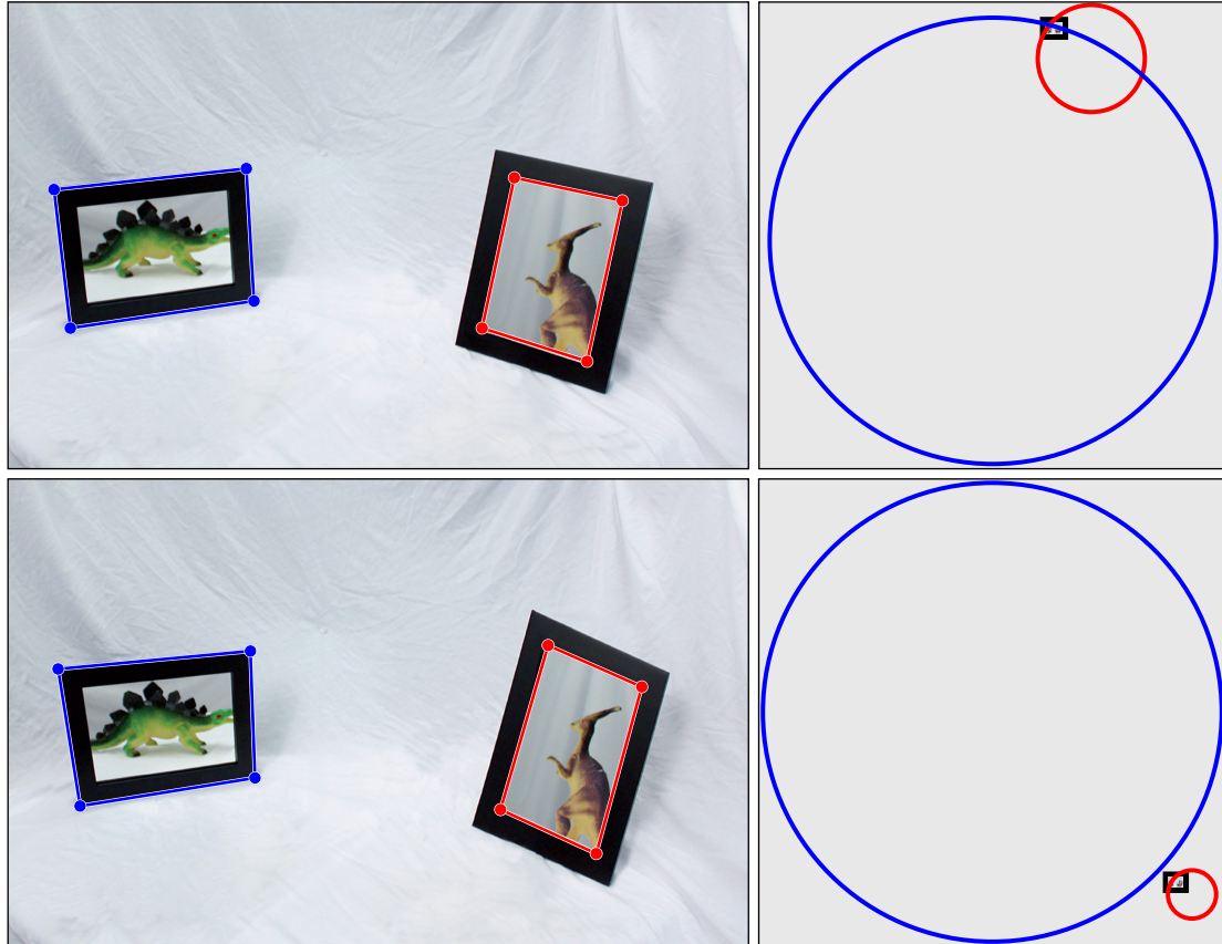
Figure 4.3: Determining the consistency of the center of projection using partial constraints. In practice, reflections are often not present in photos (top left), but are required by O’Brien and Farid [186] to estimate the center of projection. Partial constraints on the center of projection can however be specified using the pair of vanishing points that is provided by the edges of the frames (blue, red). Specifically, the center of projection can be constrained to a sphere for each frame. Each sphere is bisected by the image plane, and specifies a circle (top right). (See also Figure 4.1.) A plausible center of projection exists if the spheres, and thus the circles, intersect. Shown in the bottom row is a falsified photo in which the frames have been warped. Although this change is visually subtle, the circular constraints specified by the frames (red, blue) do not intersect (right). Furthermore, a perturbation analysis does not yield overlapping circles. We therefore correctly determine that the photo has been falsified. Photo content is due to O’Brien and Farid [186], and is modified here for illustration.
