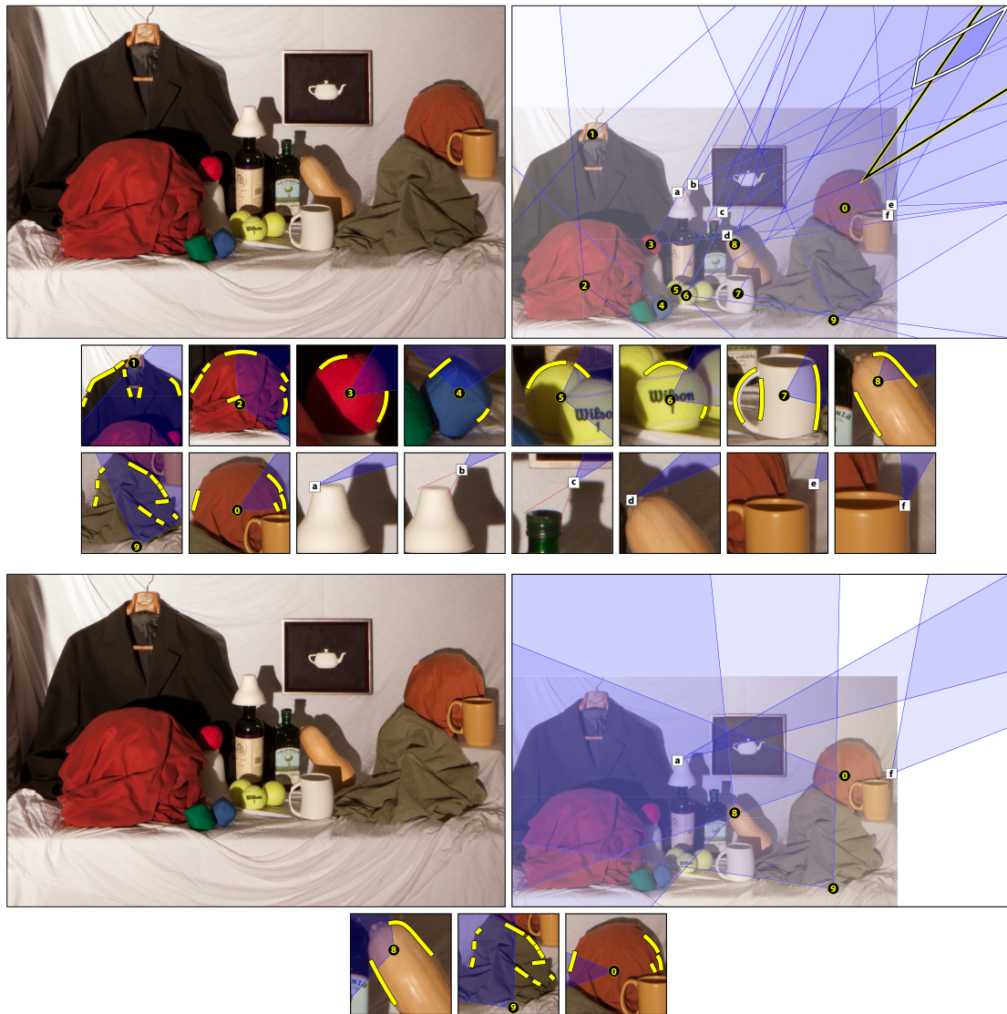
Figure 3.8: A complete shading and shadow analysis of an authentic (top) and composite (bottom) photo. Top: shading constraints, denoted by black dots, are selected from a variety of occluding contours each outlined in yellow. The outlined black region is the common intersection of these constraints, showing that they are all mutually consistent. Shadow constraints are denoted by white squares. The outlined white region is the common intersection of these constraints, showing that the shadows are mutually consistent. Because the viable shading and shadow regions intersect, the lighting in this photo is physically plausible. Bottom: in this composite photo three objects with different lighting were inserted (the squash and the green and orange shirts). The five constraints shown in the lower right are inconsistent, revealing this photo to be a composite.
