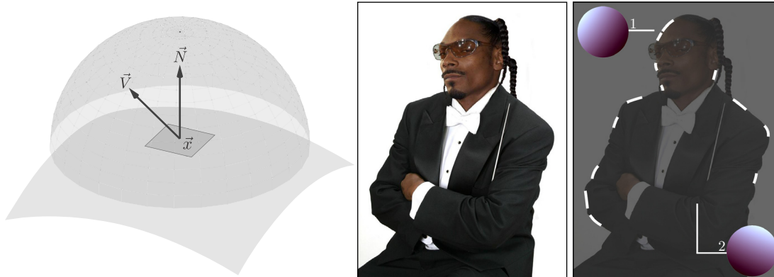
Figure 1.7: Lighting properties may be perturbed when photos are modified. Left: the brightness of a patch \vec{x} on a Lambertian surface depends upon the amount of light that strikes the patch from all directions \vec{V} on a hemisphere centered about the surface normal \vec{N} of the patch. The lighting can therefore be described as a function over the surface of a hemisphere. Middle: a falsified photo. Right: surface normals on the occluding contour (white) of objects can be used to estimate 2-D components of the lighting function. Shown is the lighting for the subject’s head and body (spheres 1 and 2). Differences in lighting evidence forgery. Figure due to Johnson and Farid [107].
