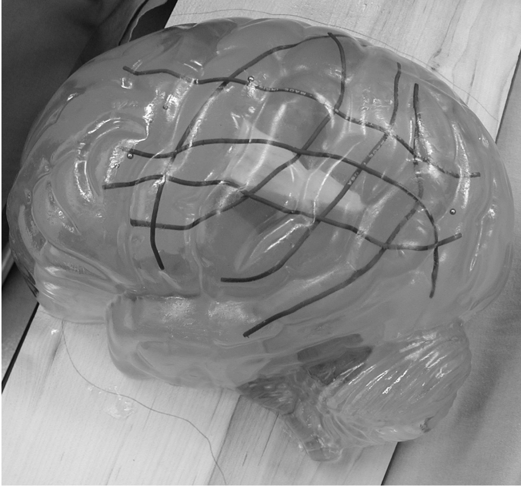
Figure 3.13: Shown is the brain phantom used to quantitatively evaluate the accuracy of the iSV system in capturing the shape of the cortical surface. Electric wires were embedded in the phantom to simulate cortical vasculature.
