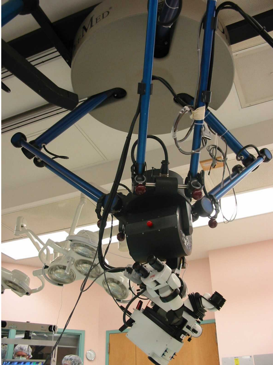
Figure 1.2: Stereoscopic operating microscope ceiling-mounted on a robotic platform.
