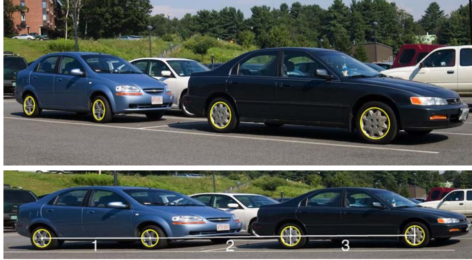
Figure A.3: The top image was rectified using four circles (wheels). Shown below is the rectified image from which the distance between the cars can be measured.
