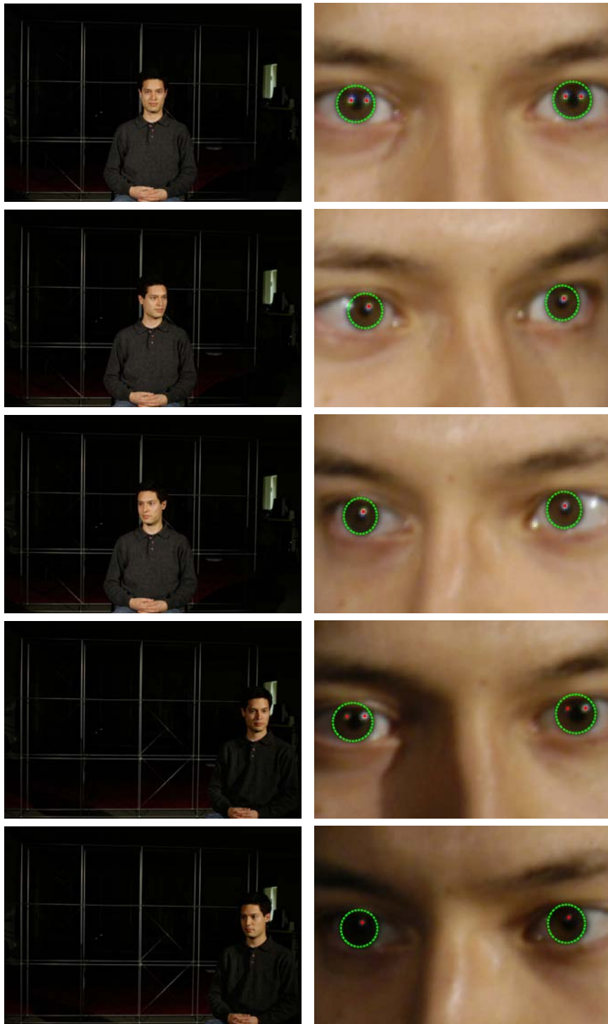
Figure 3.6: A subject at different locations and orientations relative to the camera and two light sources (left) with magnified views of the eyes (right). The ellipse fit to each limbus is shown in dashed green and the red dots denote the positions of the specular highlights. See also Table 3.1.
