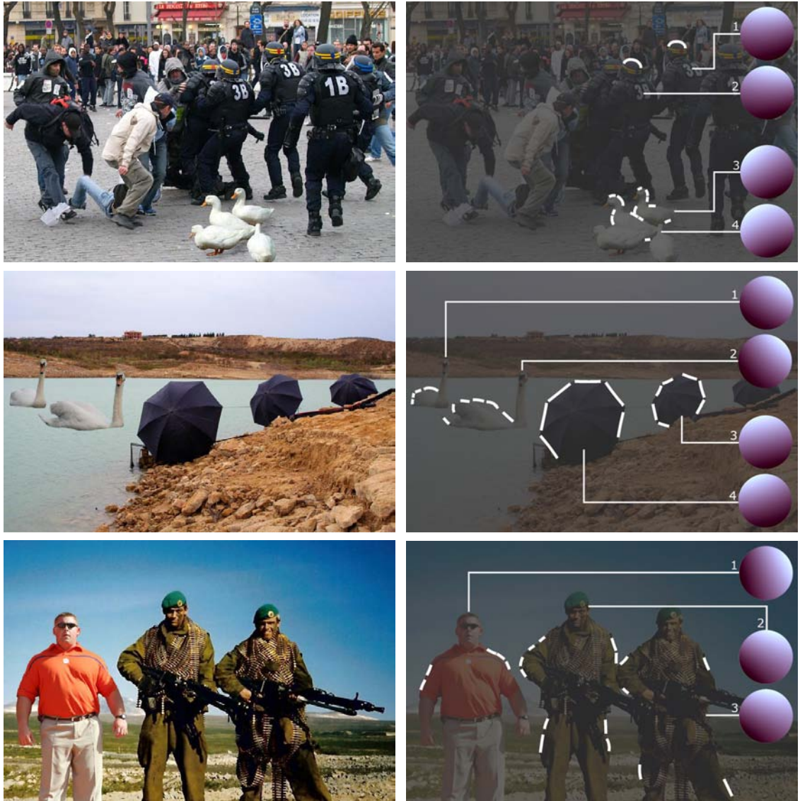
Figure 4.12: Shown on the left are three forgeries: the ducks, swans, and football coach were each added into their respective images. Shown on the right are the analyzed regions superimposed in white, and spheres rendered from the estimated lighting coefficients (see also Table 4.2).
