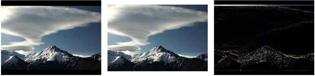
Figure 1. Shown from left to right are an original thumbnail generated by a Nikon D200, a thumbnail of the same image generated by Adobe Photoshop CS3, and the difference between these thumbnails. The Nikon thumbnail is 160 \times 120 pixels in size, while the Photoshop thumbnail is 160 \times 107 . In addition these JPEG encoded thumbnails employ different cropping boundaries and quantization tables leading to further differences as can be seen in the right-most panel.
