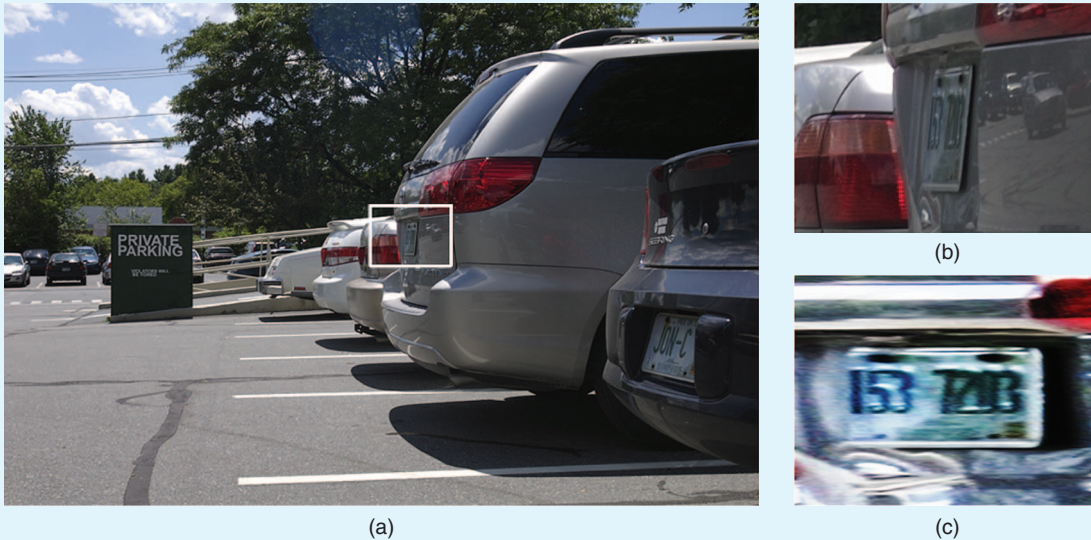
[FIG5] (a) The original image. (b) A close-up of the license plate, which is largely illegible. (c) The result of planar rectification followed by histogram equalization.
