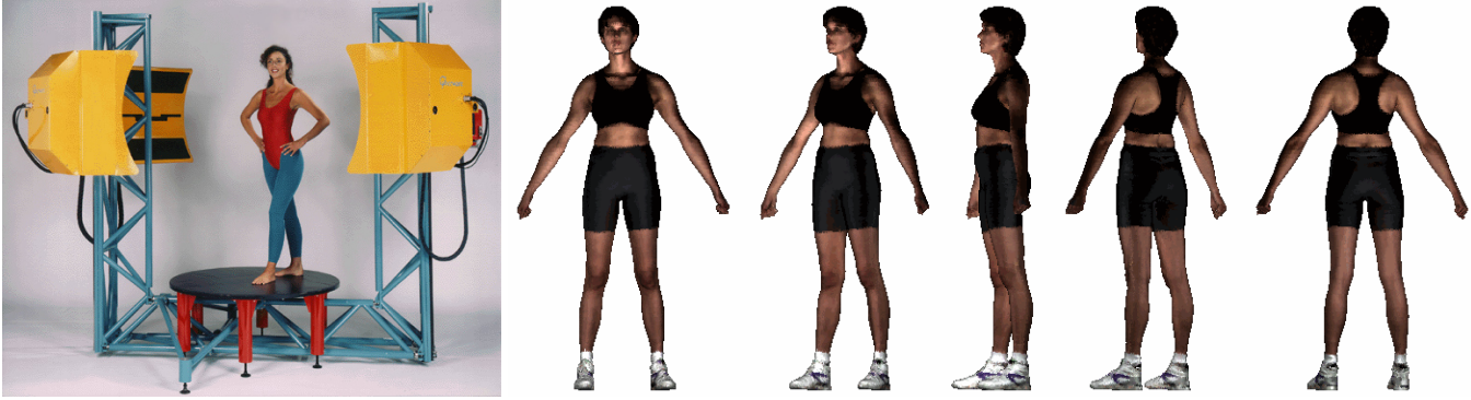
Figure 7: The whole body 3-D scanner by Cyberware and five views of a full-body scan.
