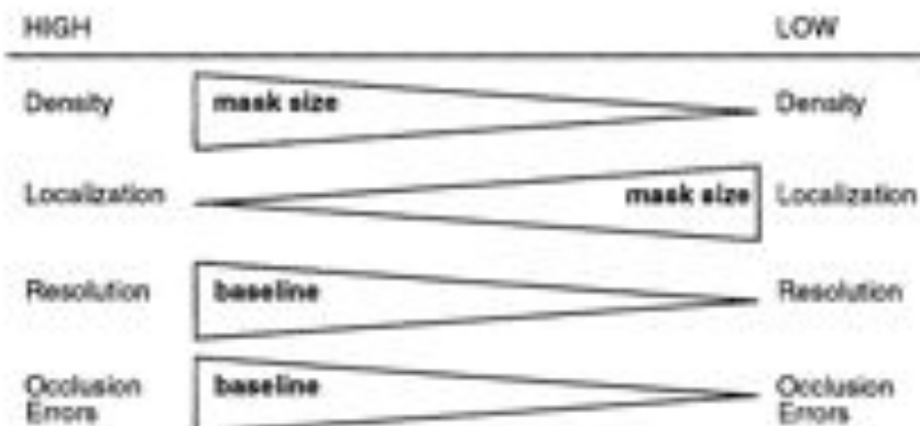
Figure 1: Tradeoffs between the baseline (distance between successive views) and the mask size (size of sampling neighborhood in which feature matching is performed). For example, a large mask size results in high density but low localization.
