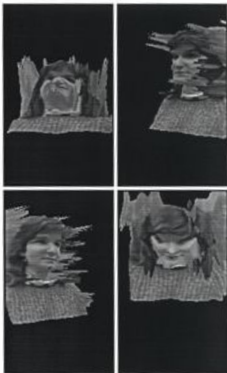
Figure 10: Depth map from our implementation of Kanade's multi-baseline algorithm. Correlation was performed on the left-most image in a 5 image sequence using a 9 \times 9 mask.
