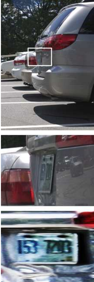
Figure 5.2 A an original photo (top), a magnified view of the license plate (middle), and the planar rectified license plate (bottom).
