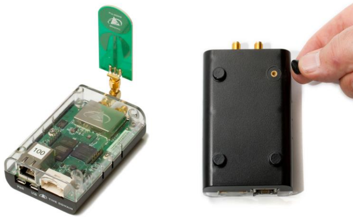
Fig. 26: P440 in standard enclosure (left) and view of enclosure bottom showing feet and mounting holes for 4-40 screw
