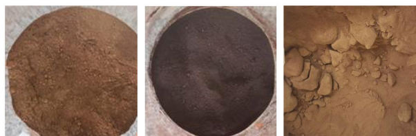
Figure 3: Photographs of lignin used in this work; crude-HKL (C-HKL, left), acetone soluble-HKL (AS-HKL, middle), and LS (right)
