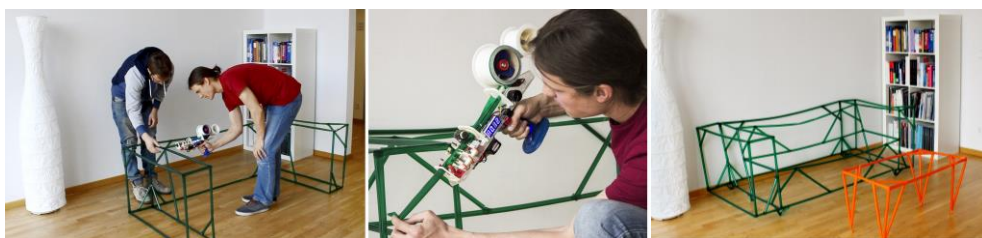
Figure 2: Protopiper is a computer-aided, hand-held fabrication device that allows users to sketch room-sized objects at actual scale – however, only for visual purposes.
