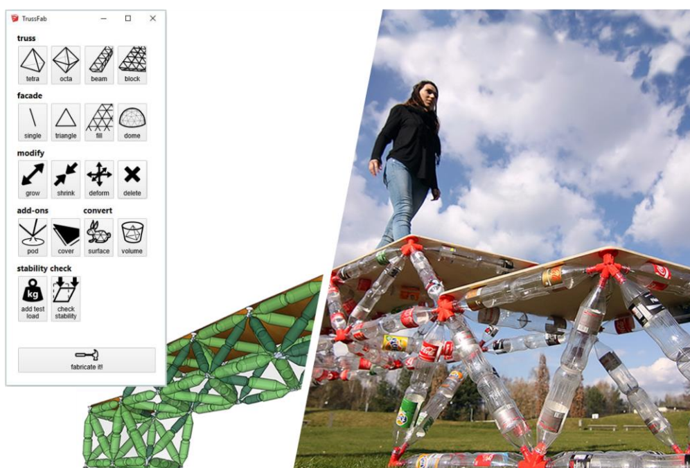
Figure 5: TrussFab is an end-to-end system that allows users to fabricate large structures sturdy enough to carry human weight. TrussFab considers bottles as beams that form structurally sound node-link structures also known as trusses , allowing it to handle the forces resulting from scale and load.
