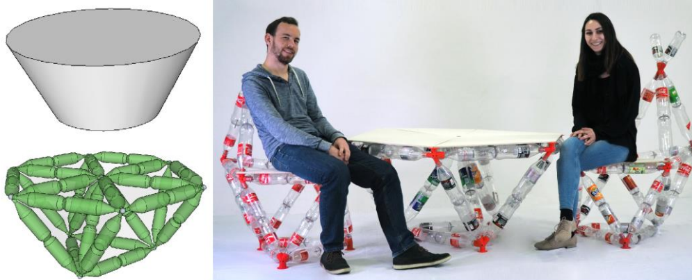
Figure 6: (a) TrussFab’s converter automatically turns this 3D model of a coffee table, into (b) a sturdy tetrahedral honeycomb structure, (c) which fabricated serves as a functional table.
