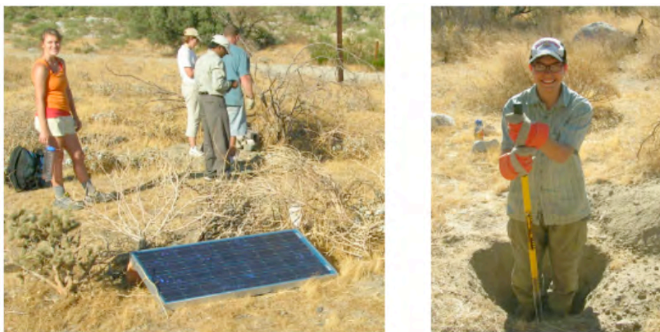
Figure 14. (Left) students working to conceal the location of seismometer and solar panels using tumbleweeds. (Right) A sizeable hole dug for one of the sensors deployed along the array.
