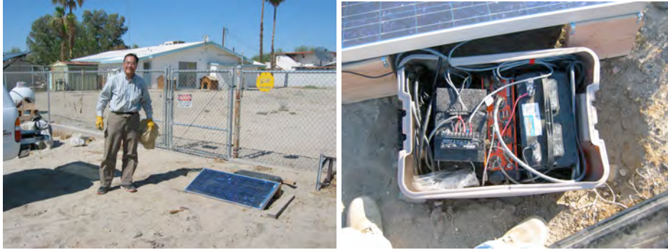
Figure 4. Joint SCEC/PASSCAL ShakeOut deployment in 2008. Installation of the SCEC PBIC real-time equipment at the [Left] Indio site with SCEC researcher Yong-gang Li shown for scale, and WWC0 center station [Right] at Whitewater Canyon.
