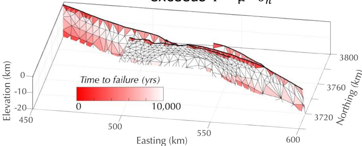
Failure when element exceeds 3 MPa
