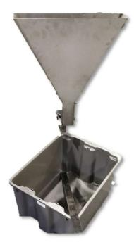
Figure 1-5: Appareil V-Funnel
