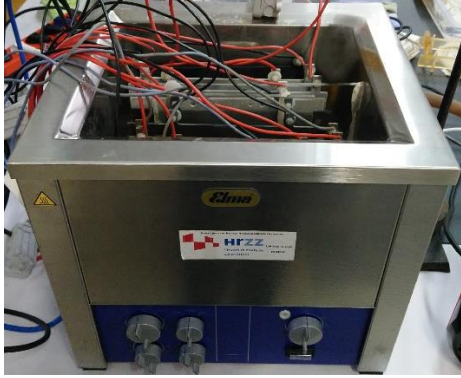
Figure 1. US bath modified as an EC reactor
