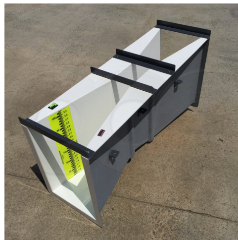
Figure 2. Parshall flume measuring structure, uninstalled [3].
