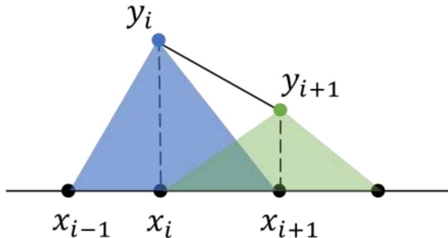
定义基函数  $B_i(x) = \begin{cases} \frac{x-x_{i-1}}{x_i-x_{i-1}}, & x \in [x_{i-1}, x_i] \\ \frac{x_{i+1}-x}{x_{i+1}-x_i}, & x \in [x_i, x_{i+1}] \\ 0, & \text{else} \end{cases}$
