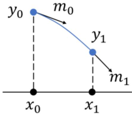
$$y = \overset{h_{00}}{(2t^3 - 3t^2 + 1)}y_0 + \overset{h_{10}}{(t^3 - 2t^2 + t)}m_0(x_1 - x_0) + \underset{h_{01}}{(-2t^3 + 3t^2)}y_1 + \underset{h_{11}}{(t^3 - t^2)}m_1(x_1 - x_0)$$
