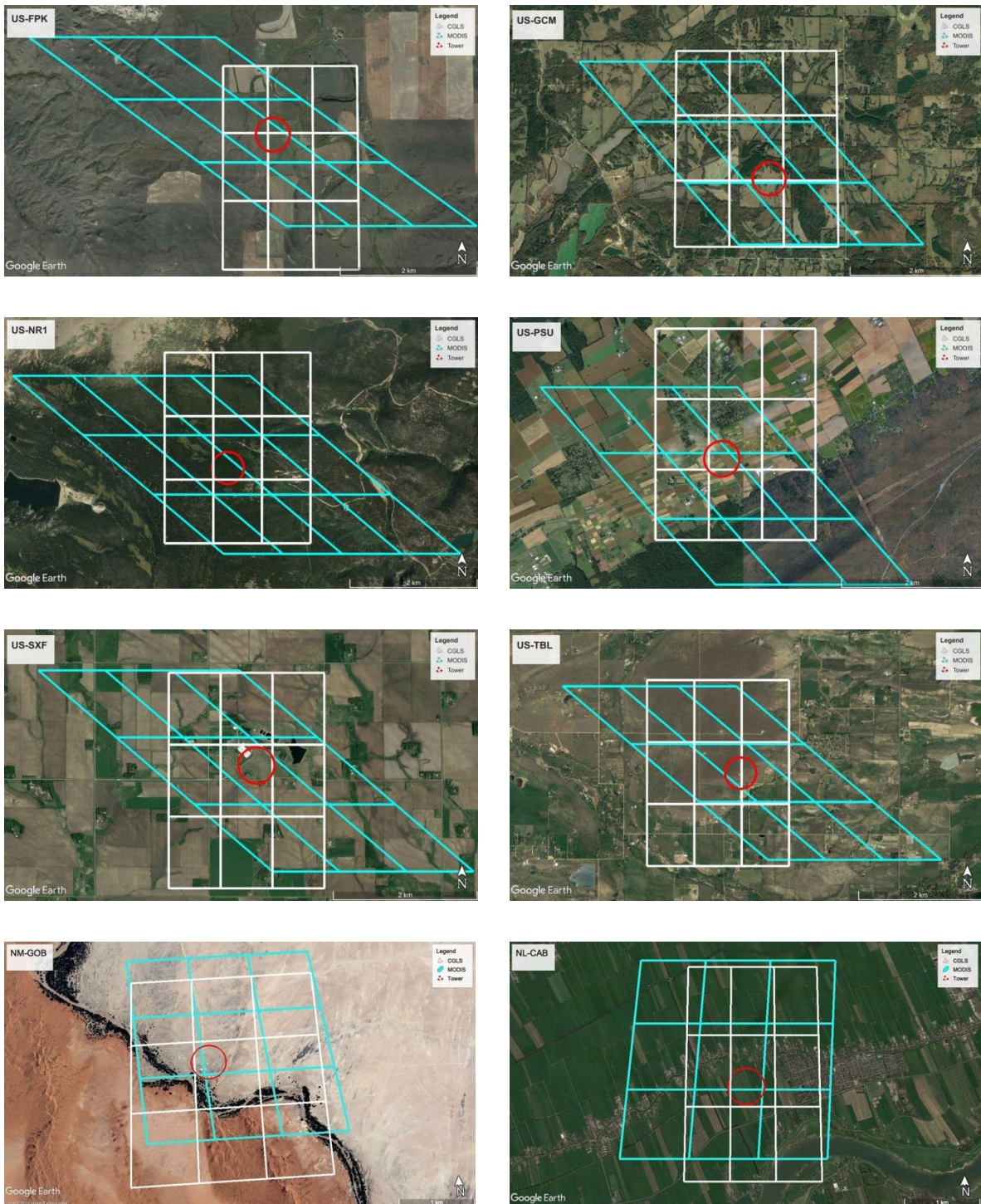
Figure 3. Overview of selected tower sites (taken using Google Earth). The white line represents CGLS Spot/VGT product pixel footprints of 1/112^{\circ} , the MODIS SIN projection grid for 3 x 3 km pixels is shown in cyan and the red circle around the tower shows a 500m radius equivalent to a tower albedometer footprint from a tower of 50m in height. The site short-name is indicated and a nadir view employed. No standard VGT-CGLS data are produced above \pm 60^{\circ} of latitude so neither BSRN-BRW nor SPO are displayed. N.B. The MODIS SIN projection is more distorted in the Western hemisphere, the further the west one goes.
