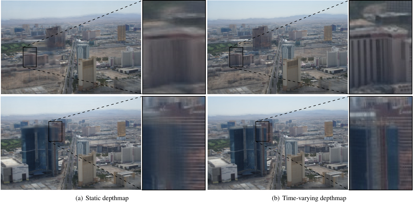
Figure 8. Comparison of output time-lapse frames for two different timestamps for the Las Vegas sequence. a) Using a static depthmap solved with a discrete MRF as in [12]. b) Using our time-varying, temporally consistent depthmaps. The static depthmap is not able to stabilize the input images for the whole time-lapse, creating blurry artifacts where the geometry changes significantly. Thanks to the time-varying depthmap, our 3D time-lapses are sharp over the whole sequence.
