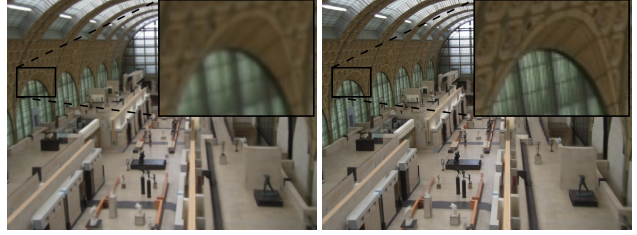
Figure 7. Comparison of two methods for output frame reconstruction from projected profiles for the Musée D'Orsay scene. Left: baseline method based on Gaussian kernel splatting, with kernel radius \sigma = 1 . Right: our reconstruction approach. The baseline method produces a blurred reconstruction, whereas the proposed approach recovers high frequency details in the output frame.
