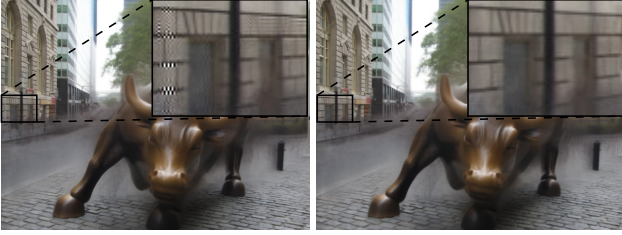
Figure 6. Comparison of different values of the 3D track sampling threshold \epsilon for the Wall Street Bull scene. Left: Artifacts are visible when \epsilon = 1 pixel, with alternating black and white pixels, as the reconstruction problem is badly conditioned. Right: Using \epsilon = 0.4 pixel, the artifacts are not present.
