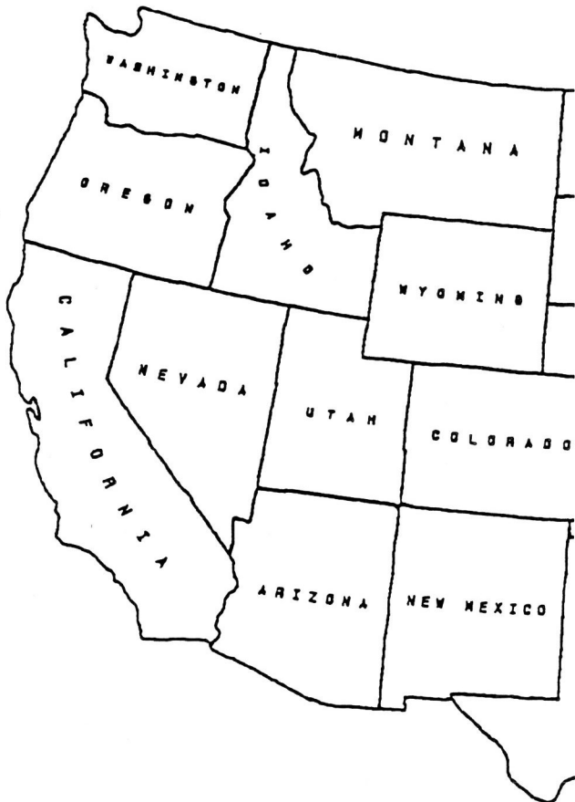
Fig. 3. Example of area-feature name placement. (The placement was done by the program described here, without human intervention.)
