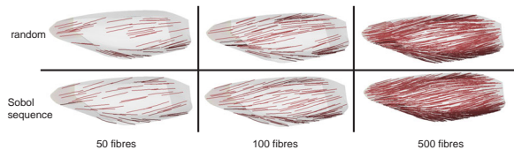
Figure 7: Generation of fibres. 50, 100, and 500 fibres were generated in a model of the posterior soleus using uniform pseudorandom number generation and Sobol sequences. The Sobol sequence produced better distribution of fibres.
