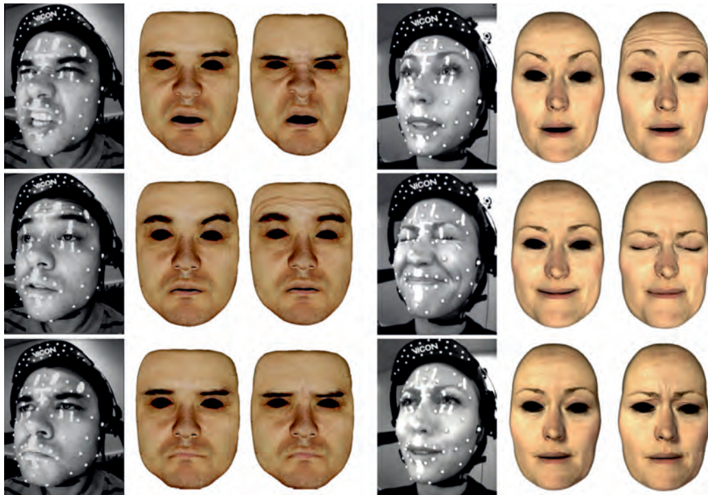
Figure 9: Animation Results: The left-most image of each 3-tuple shows an example image from our HMC. Middle images show results using only markers. The right images show results using markers combined with video classification. Our method is able to capture subtle motions between the eyes such as AU 9 (top-left tuple) and AU 4 (bottom row) which are missed when using only markers. This drastically changes the way the facial expression is perceived. Also increased control over blendshape selection allows us to detect when wrinkles should show up (top-right and center-left tuples)
