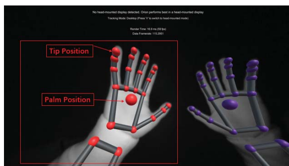
Fig. 4. The interface of Leap Motion
